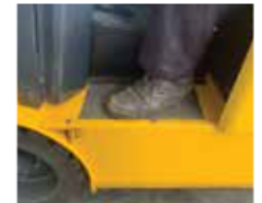
Wider Operator foot rest for safer entry and exit
