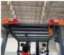
High Mounted Rear Combination and Beacon Lights
