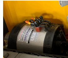
Rear mounted hoist motor for easy maintenance
