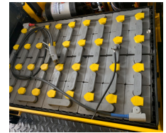
72V battery & AC traction for longer hours of operation
