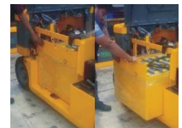
Easy side removal of battery (optional)
